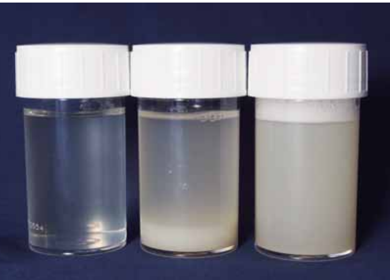
Fig. 1: Comparison of the preparation of gelatine (left) compared to FloraClair® without mixing (middle) and after gentle mixing (right) just before use. © all photos Erbslöh
